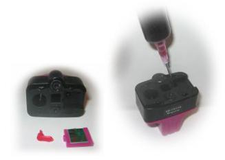
Reinsert the small plastic plug back into the filling hole. Be sure that it is pushed in well and that it is positioned at seen in the picture
